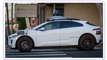
Sensors on the car let a computer steer it with no driver
