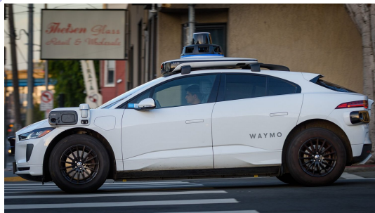
Sensors on the car let a computer steer it with no driver
