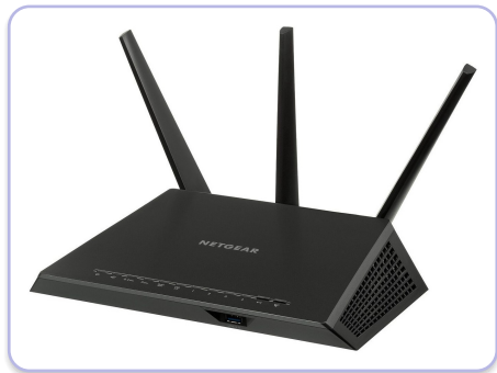
A Wi-Fi router forwards packets between networks
