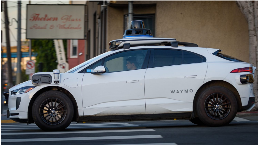
A self-driving car: sensors on the car let a computer steer it with no driver
