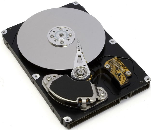
Inside a hard disk drive (HDD): the shiny disk spins and the arm reads the magnetised data
