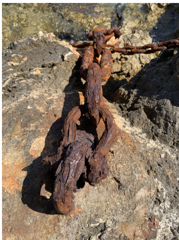
Sea water and air have badly rusted this iron chain — the rust is hydrated iron(III) oxide
