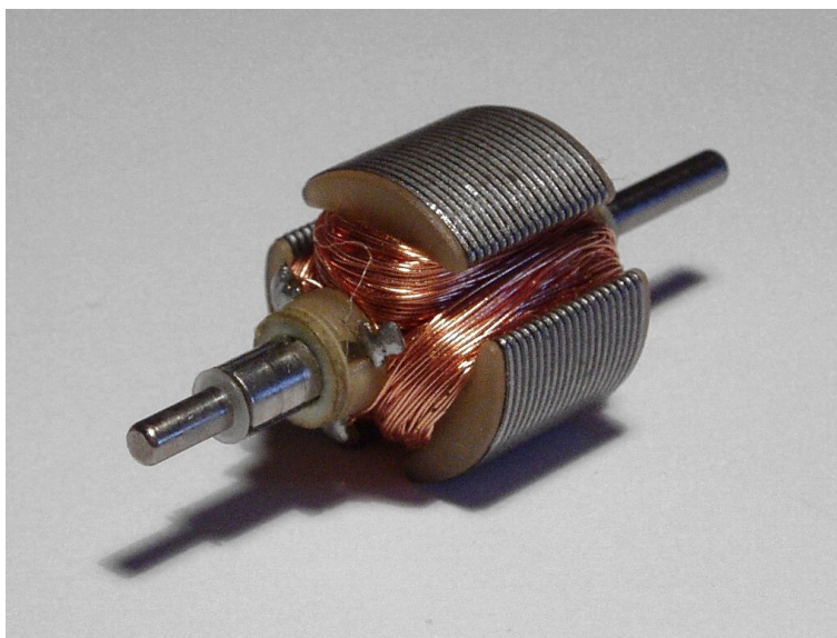
Coils of wire spinning in a magnetic field: moving them past the field induces a current, the basis of a generator
