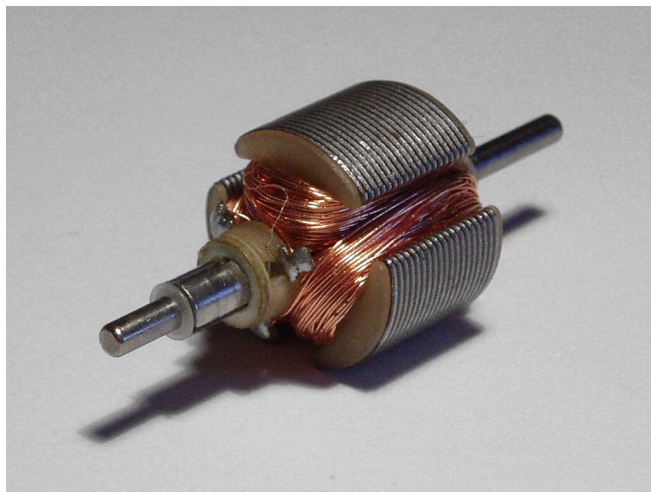
Coils of wire spinning in a magnetic field: moving them past the field induces a current, the basis of a generator
