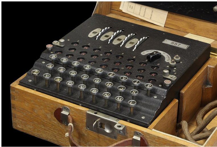
The Enigma machine scrambled messages with rotors — an early, breakable example of encryption
