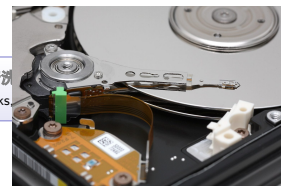
Hard-disk platters and head: data compressed and stored as magnetic patterns
