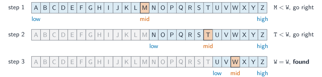
Binary search halves the range at each step (the list must be sorted)
