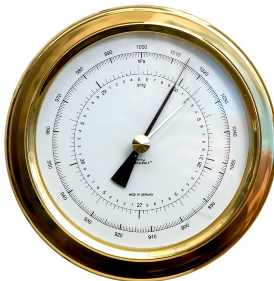
A precision aneroid barometer measures atmospheric pressure
