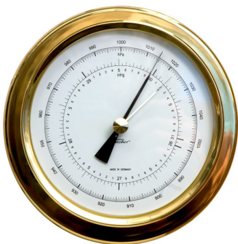
A precision aneroid barometer measures atmospheric pressure
