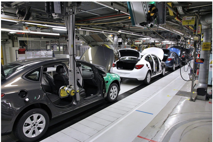
A car assembly line: capital (machines and robots) plus the division of labour, each worker repeating one task.
