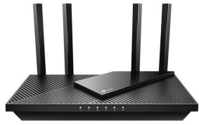
A home Wi-Fi router: it forwards packets between your devices and the internet
