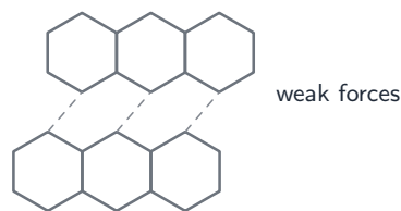
graphite layers slide; spare electrons let it conduct
