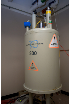
A tall cylindrical NMR spectrometer with a strong magnetic field warning
