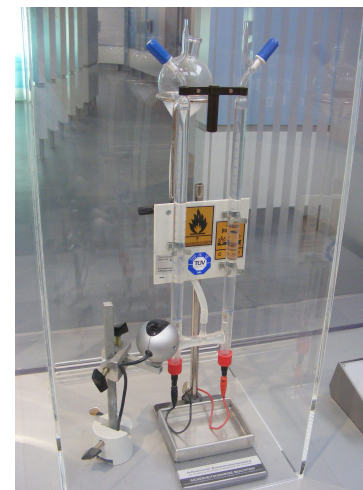
A Hofmann voltameter for the electrolysis of water: the power supply drives current through two electrodes, and the gas made at each one collects in its side tube
